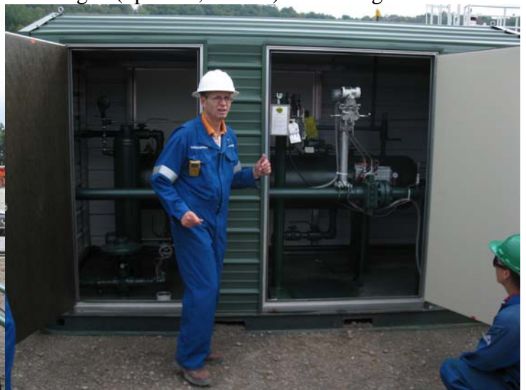
Gas "treatment" is minimal as gas is very clean, only needs dewatering and then sent to pipeline.
