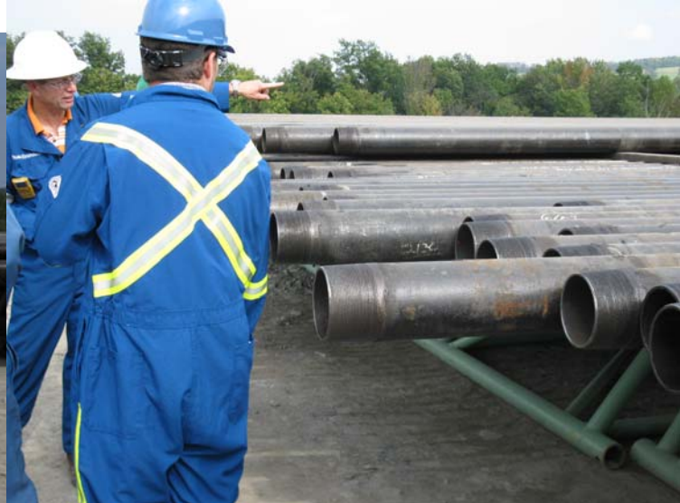
Interior well casing, very heavy gage pipe casing capable of handling 10-12,000 lbs/in2
