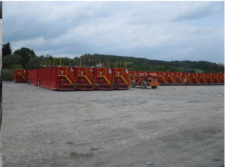
Wellhead for ready for fracing and water storage tanks on site holding just some of the water needed
