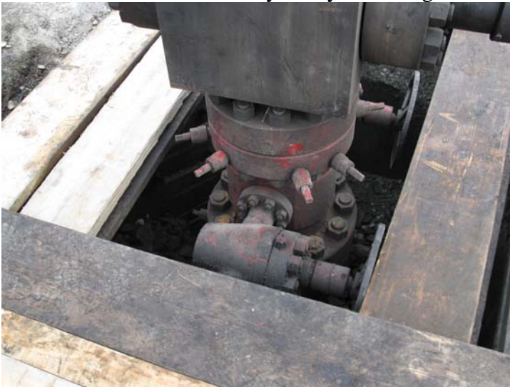
Wellhead for ready for fracing and water storage tanks on site holding just some of the water needed
