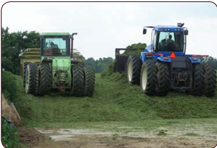
Tractors hard at work packing hay crop silage to optimize silage density.
