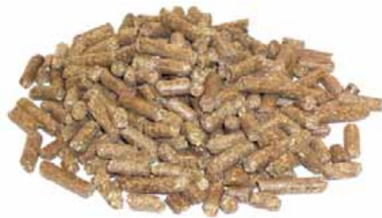
Grasses do not require any binders to form good pellets, but the pellet die and pelleting conditions need to be adjusted to grass.
